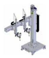
Station solution 2 is a conventional column and boom, with a movable boom and one welding head mounted at the end, combined with a boom-carriage-mounted welding head. (Not CaB 300).
