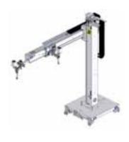
Station solution 4 is a side-boom manipulator with a double track boom. The welding heads are placed on each side of the boom. The boom carriages can be individually controlled by the joint tracking systems, on separate tracks. Positioning from the rail carriage helps to create a highly-efficient welding station for the transversal, double fillet welding of stiffeners, for example.
